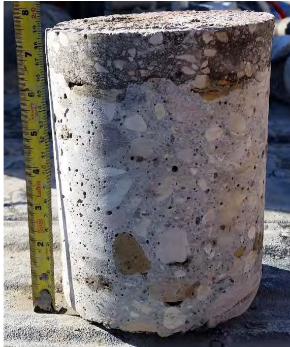
Figure 35: TH34 – 30 mm asphalt, 160 mm intact concrete
