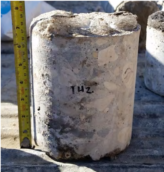
Figure 30: TH30 – 180 mm intact concrete
