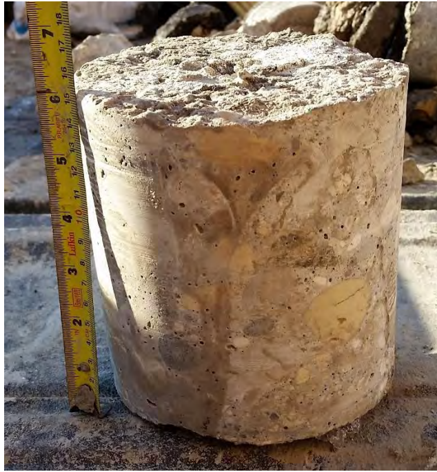
Figure 11: TH11 – 160 mm intact concrete
